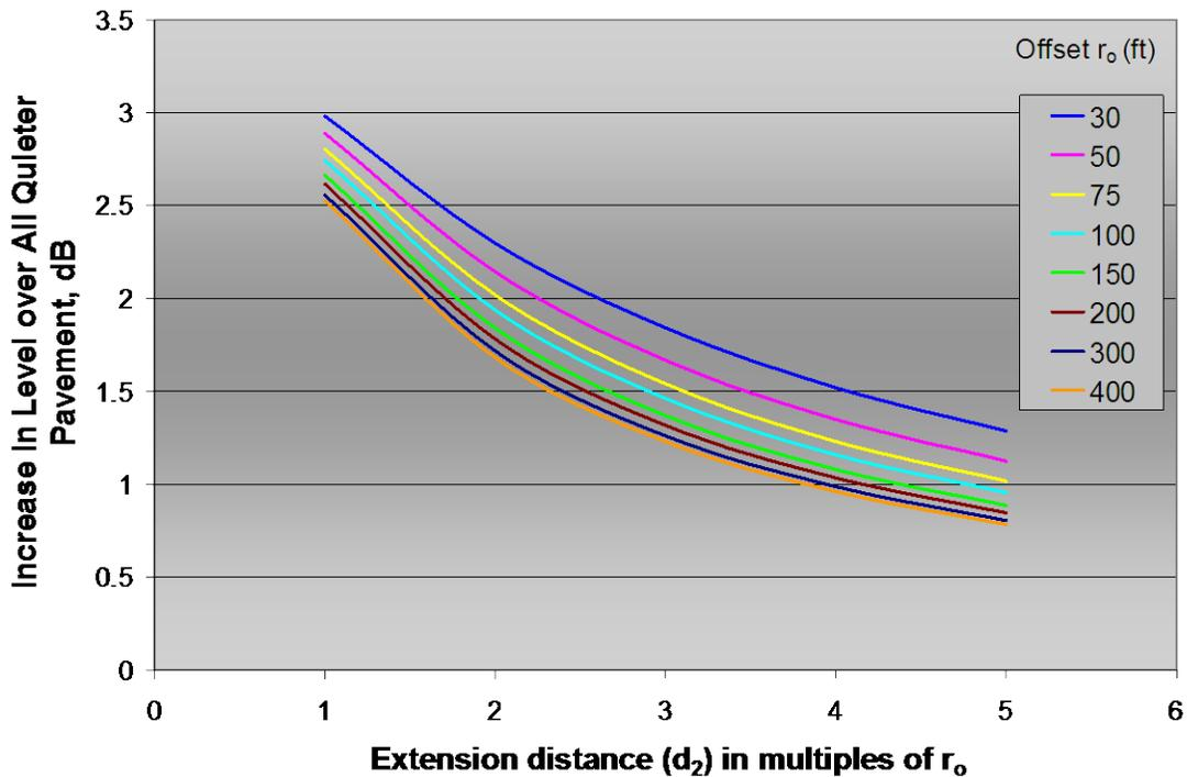
**Figure 4:** Eight Lanes Twenty Four Foot Median, 97 and 103 OBSI Levels
