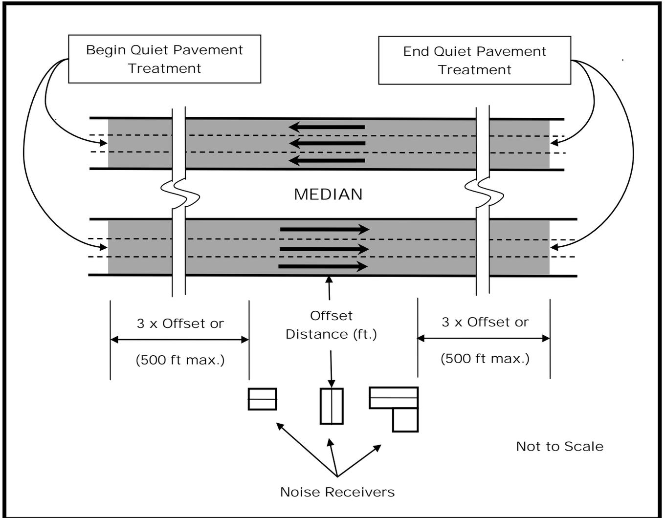
**Figure 10:** Diagram from Caltrans Quiet Pavement Policy Bulletin Defining Limits of Quieter Pavement Projects
