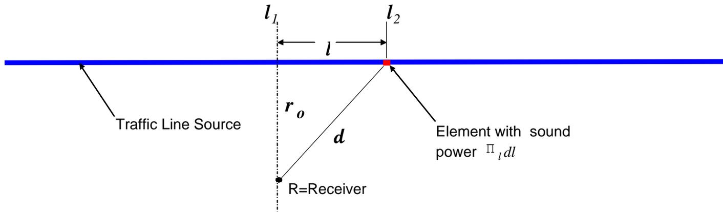
**Figure 1 :** Quieter Pavement Line Source Geometry
