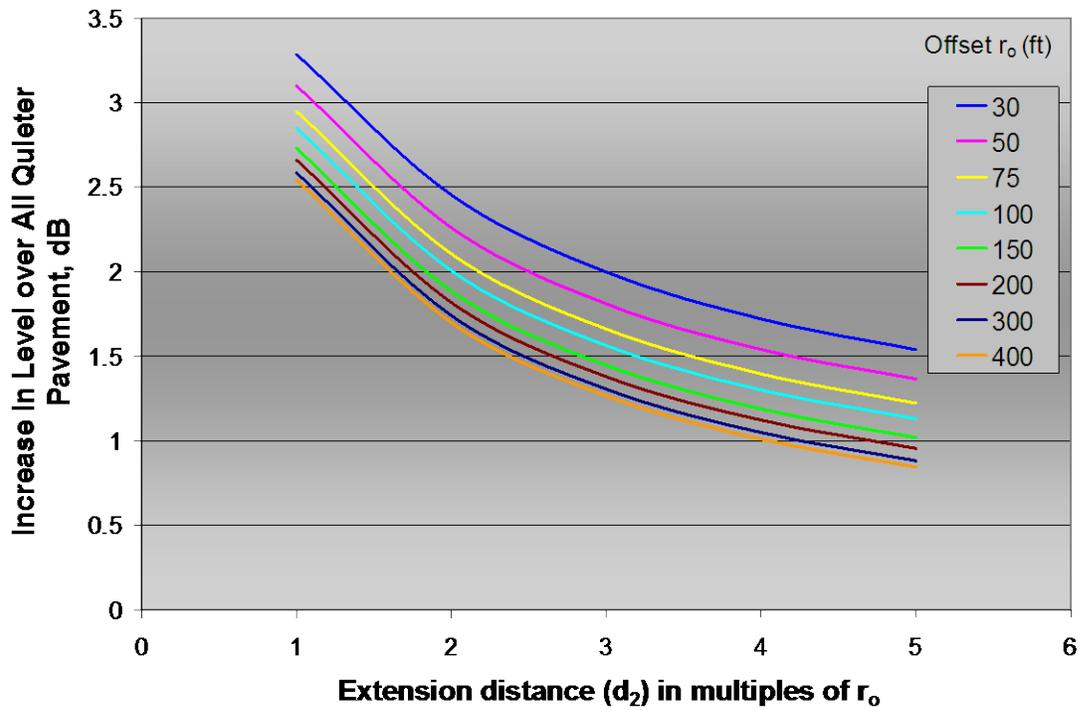
Figure 6: Two Lanes Twenty Four Foot Median, 97 and 103 OBSI Levels
