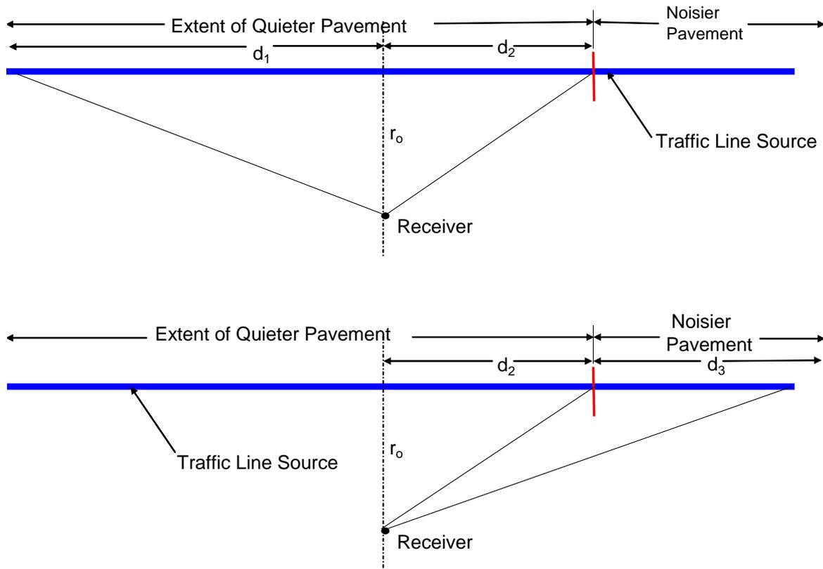
**Figure 2:** Model Geometry for Quieter/Noisier Pavement Line Source
