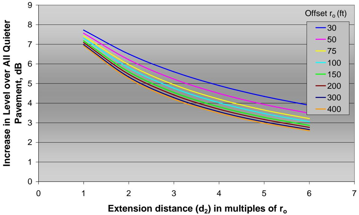
**Figure 8:** Eight Lanes Twenty Four Foot Median, 97 and 109 dB(A) OBSI Levels
