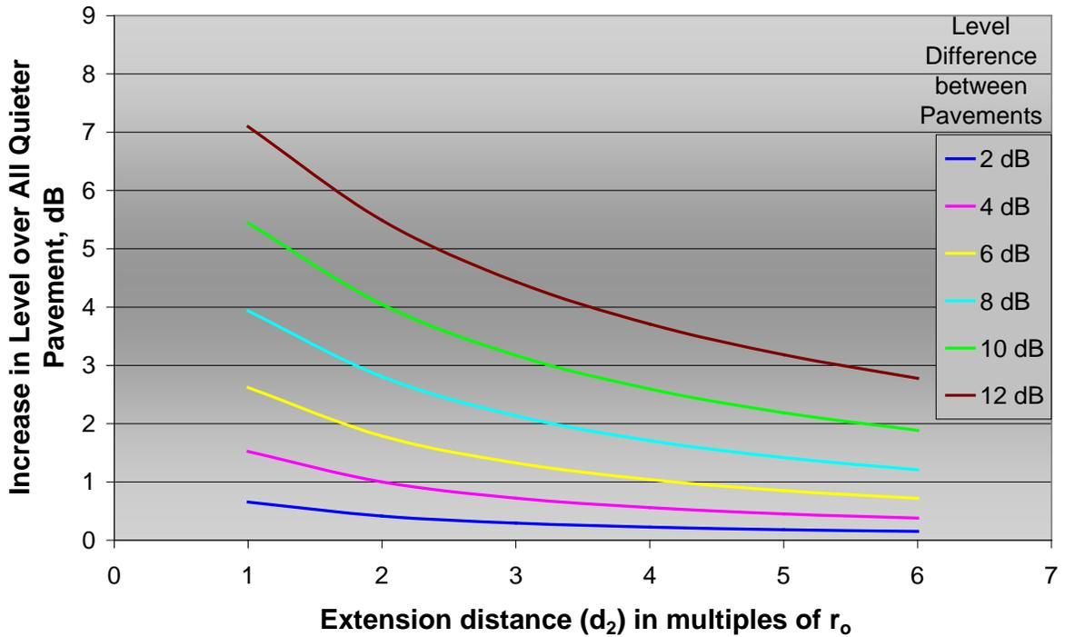
**Figure 9:** Six Lanes Twenty Four Foot Median Receiver at One Hundred Fifty Feet for Different Level Differences between Quieter and Noisier Pavement
