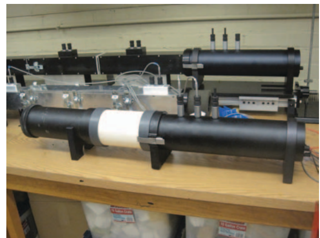
FIGURE 5 Impedance tube in test for normal incidence acoustic absorption.
