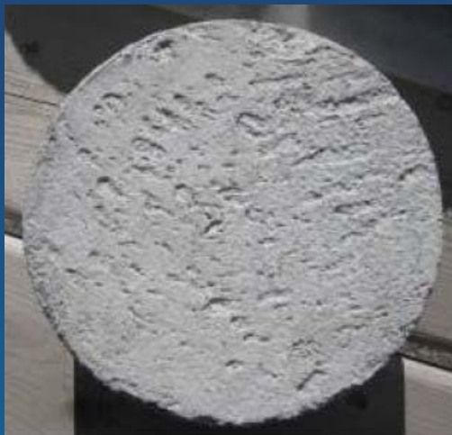
a) Screed Finish
